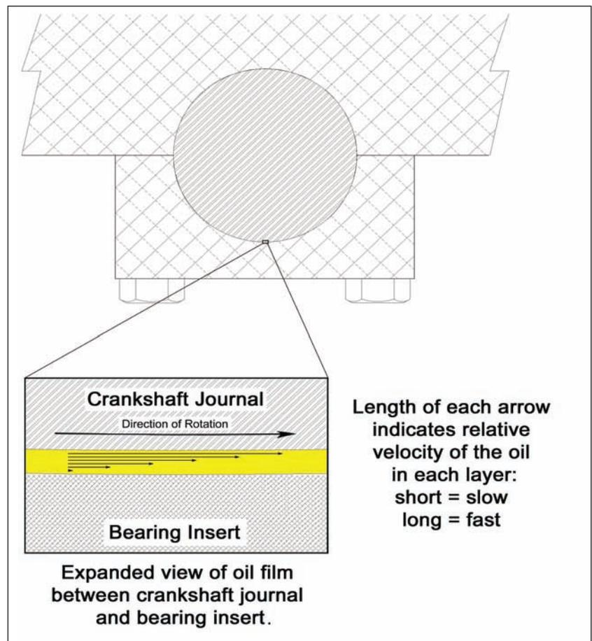
figure 10 - Oil Shear Between Moving Journal and Bearing
