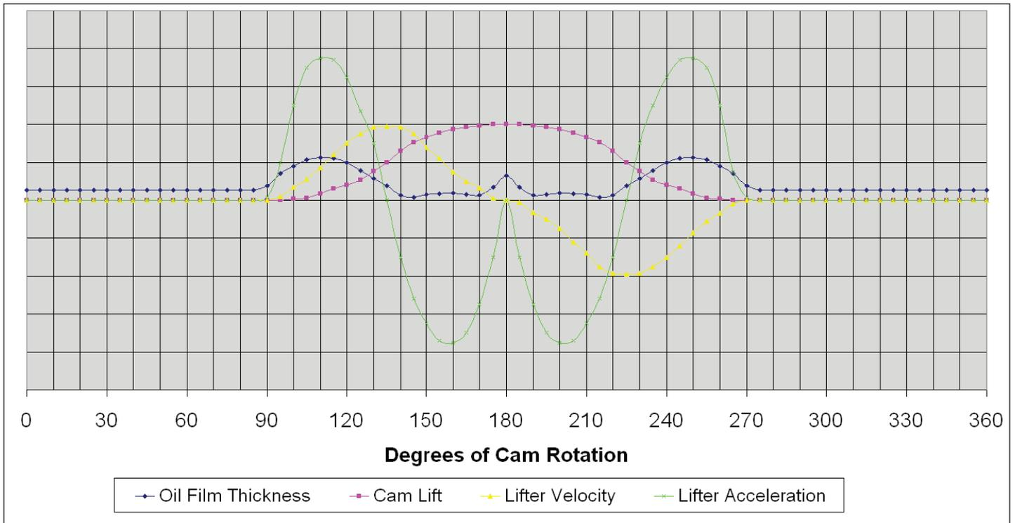
**figure 11 - Cam and Lifter Characteristics and Timing**
