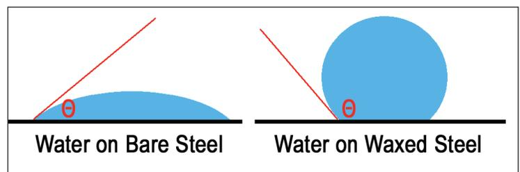
figure 6 - Polarity Affecting Adhesion
