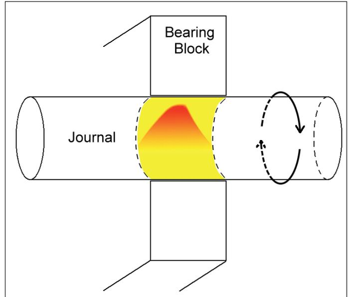
**figure 8 - Hydrodynamic Pressure Profile with Side Leakage**
