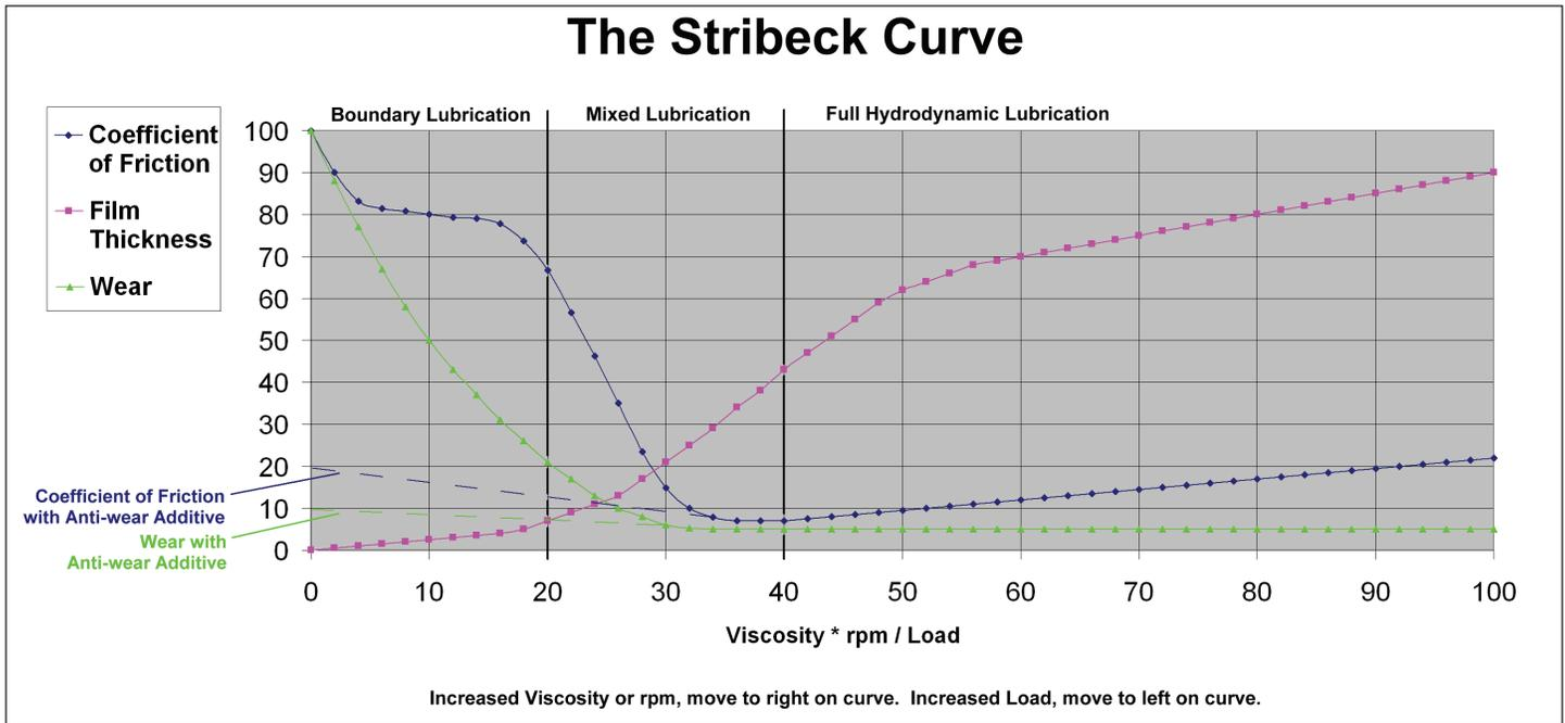
figure 2 - The Stribeck Curve (Plus Coefficient of Friction and Wear Curves)
