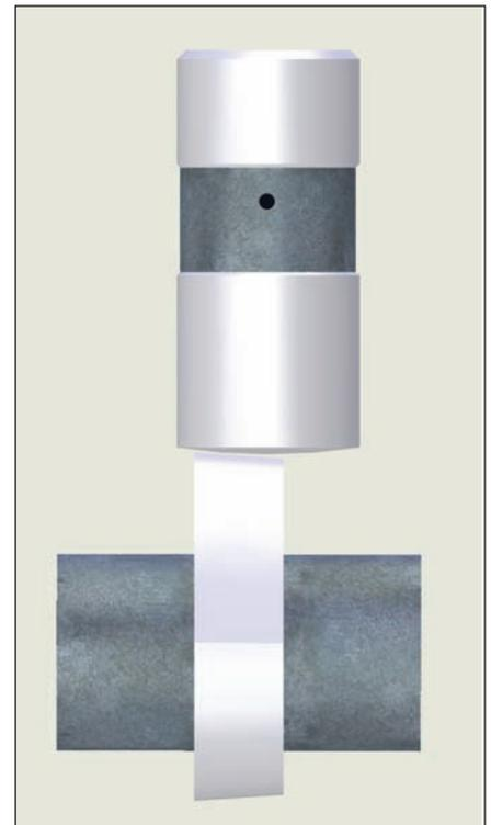
figure 12 - Ideal Cam / Lifter Contact
